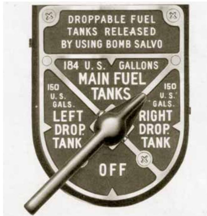
FIGURE 2: Main fuel control showing the three basic positions.
