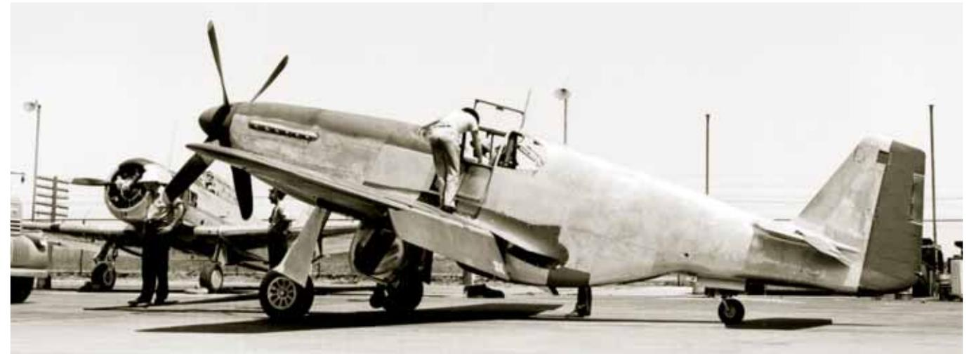
At the Dallas facility, a P-51C is prepared for its first flight test. Depending on schedules, completed aircraft were sometimes flown with incomplete factory schemes. As can be seen, this Mustang has yet to receive national insignia and other standard markings. Zinc chromate areas would be removed prior to USAAF delivery.
