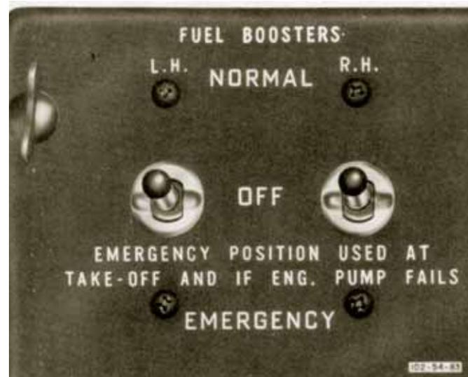
FIGURE 1: The switches for fuel booster pump operation.
