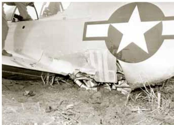
Typical crash-landing damage to the scoop area.
