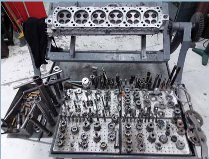
The Rolls-Royce head tool required to install the valve seats.
