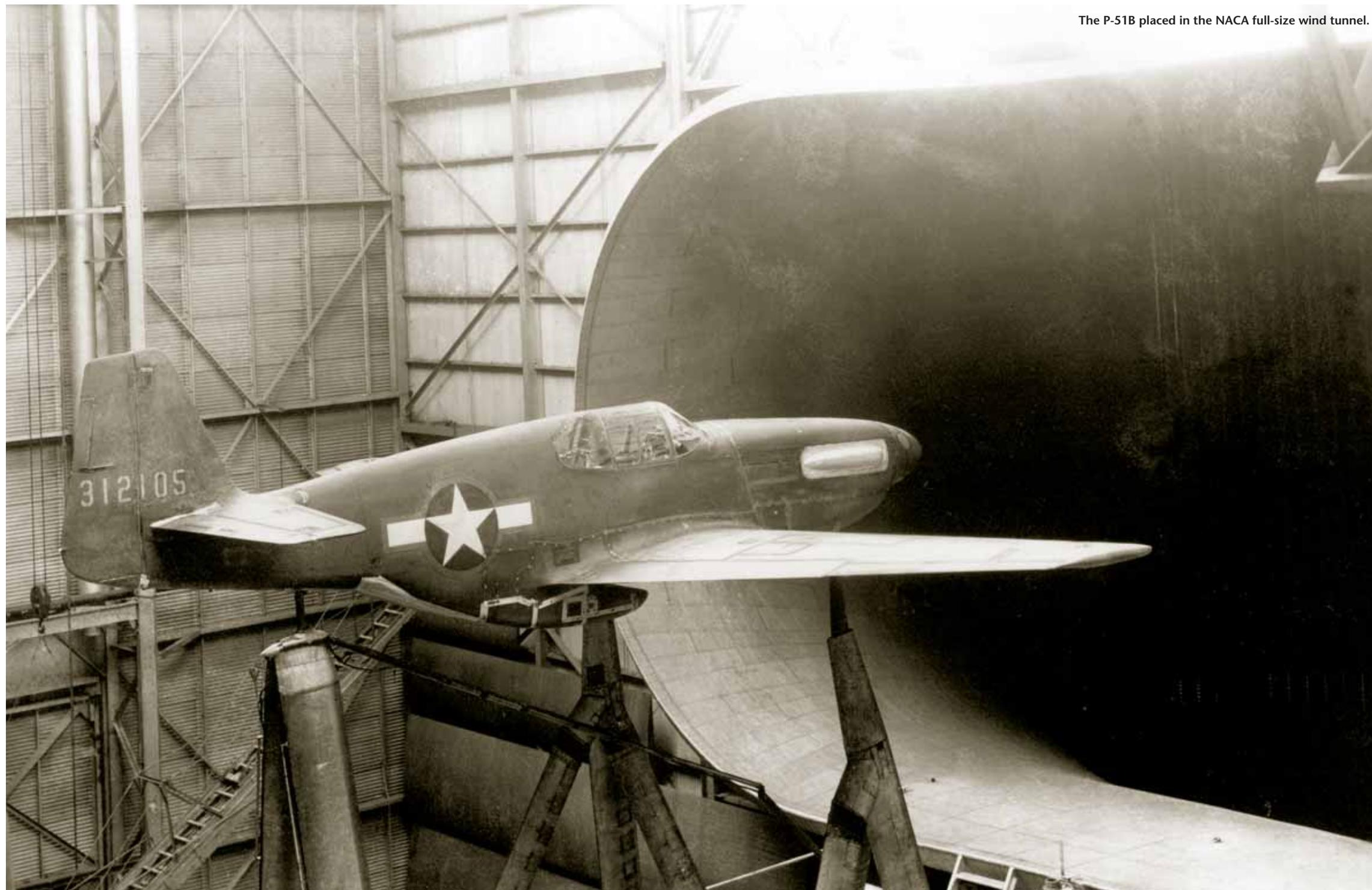
The P-51B placed in the NACA full-size wind tunnel.
