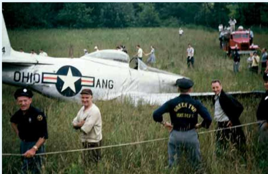
The wrecked F-51H quickly became a tourist attraction. Captain Bleimes continued, "I was trying to deal with the problems and avoid the crowd of over 100,000 people, I wound up setting it down in a field off the end of a runway. The left wing and propeller tore off, and the fuselage broke on both sides of the cockpit." Obviously time had changed his memory a bit since the fuselage was buckled not broken, and the left wing was still attached to the aircraft.
